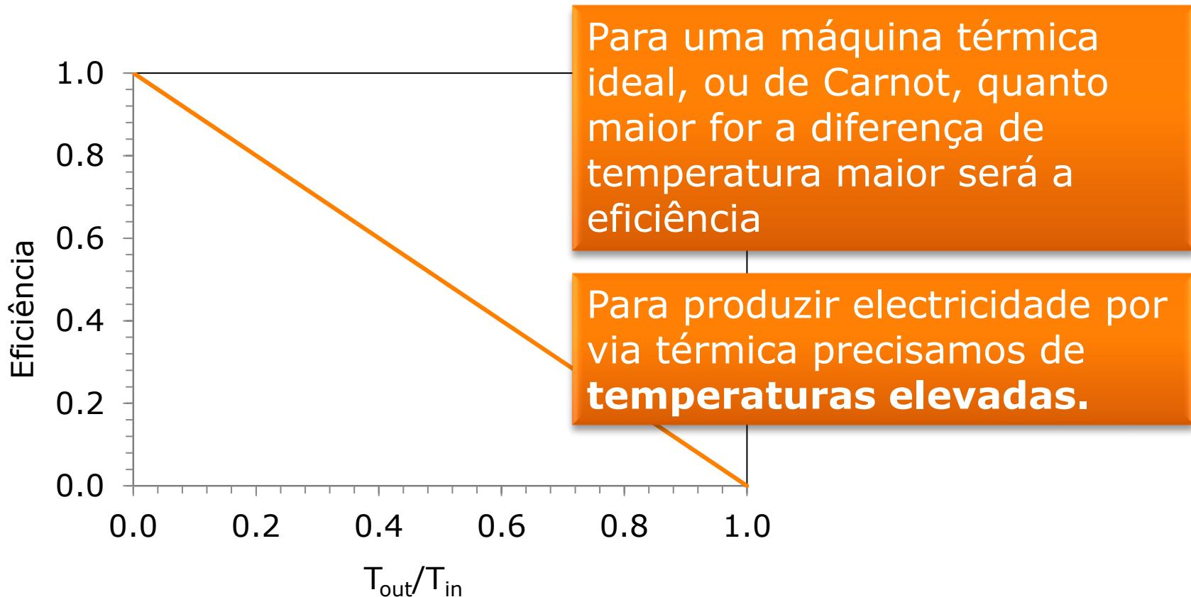
$$\eta = \frac{W_{out}}{Q_{hot}} = \frac{Q_{hot} - Q_{cold}}{Q_{hot}} = 1 - \frac{Q_{cold}}{Q_{hot}} \leq 1 - \frac{T_{cold}}{T_{hot}}$$
